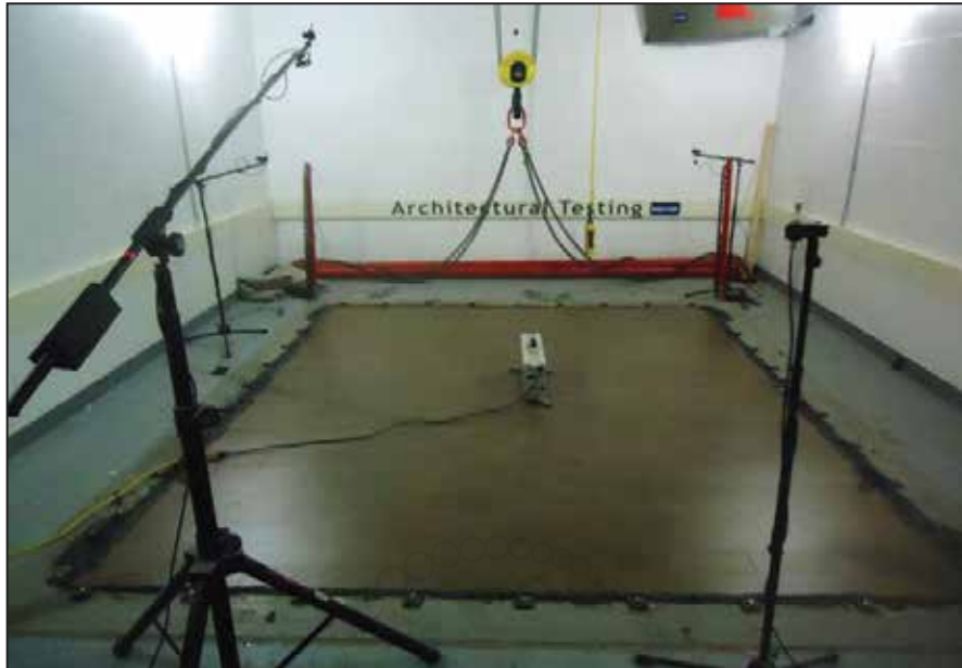
Source Room View of Test Specimen Installation
